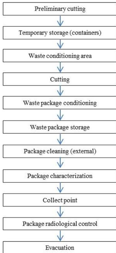
Fig. 2 Flowchart of core dismantling process
