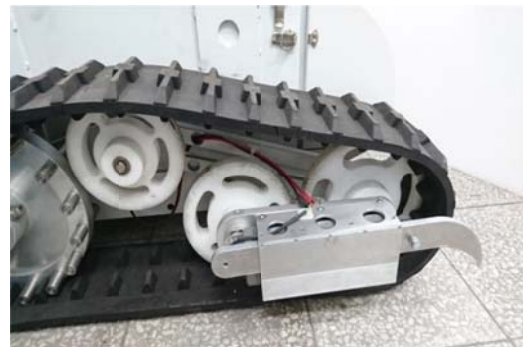
(b) A photo of track posture in the lower position
