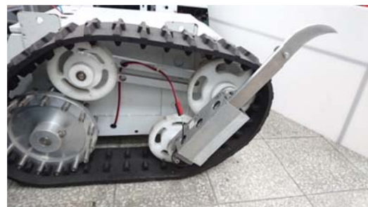
(d) A photo of track posture in the higher position
