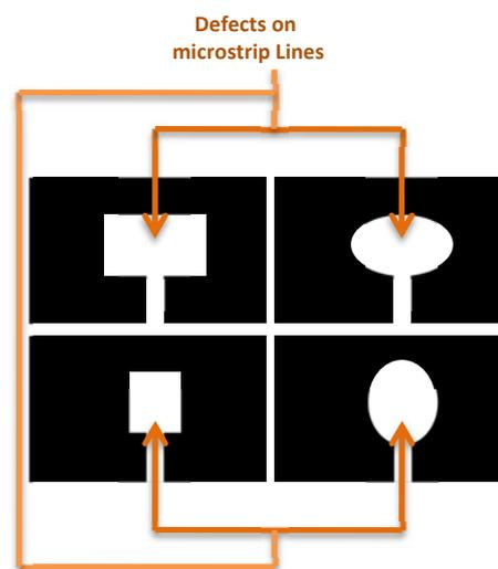
Fig. 1 Some examples of defects on Microstrip lines
