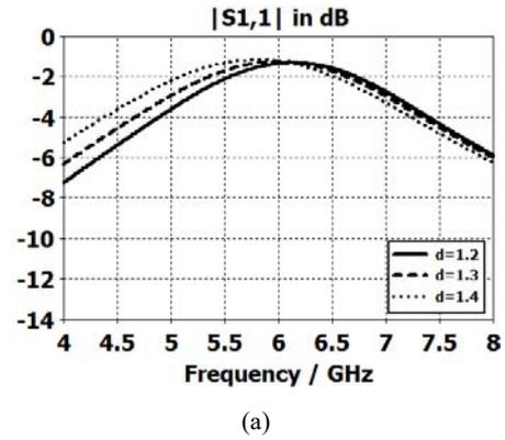
Fig. 4 Simulation of S11 (a) and S21 (b) with varied parameter a
