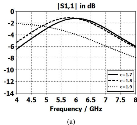
Fig. 5 Simulation of S11 (a) and S21 (b) with varied parameter b
