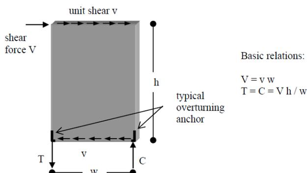
Fig. 1 Illustration of the transmission forces principle [1]
