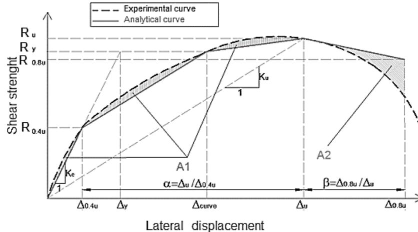
Fig. 3 Multi-linear model for shear wall force-displacement curve
