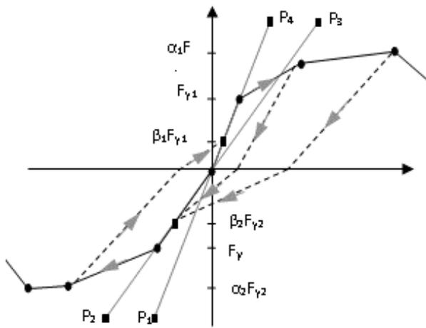
Fig. 4 Multi-linear plastic pivot hysteresis model principle [9]
