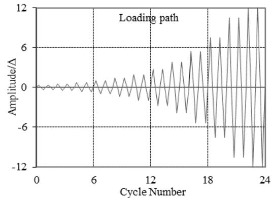
Fig. 5 CUREE reversed cyclic test protocol
