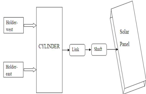
Fig. 4 Schematic layout of Solar tracking system
