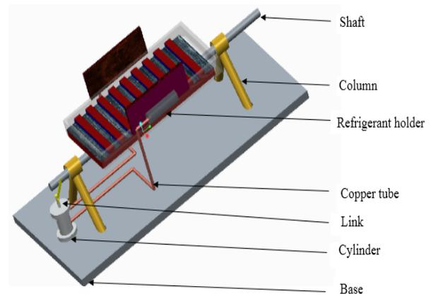
Fig. 5 Model of Solar Tracking System with Refrigerant
