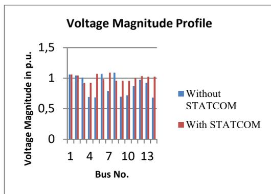
Fig. 8 Voltage magnitude profile with and without STATCOM
