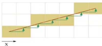
Fig. 3 Incremental line drawing by DDA
