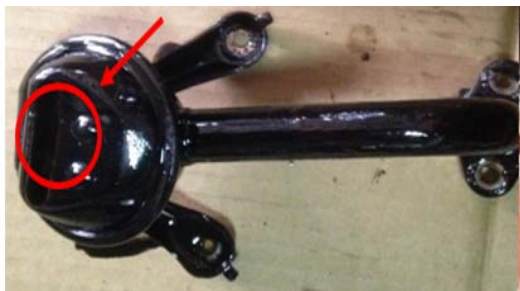
Fig. 5 Contaminates and sludge accumulated on the oil filter
