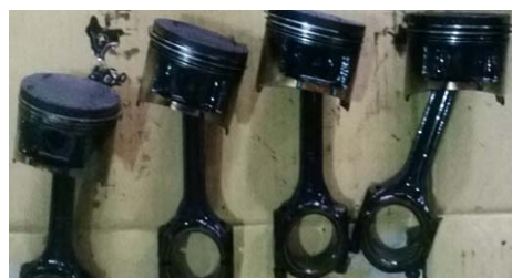
Fig. 8 Disassembled pistons and connecting rods
