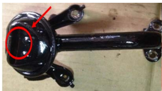
Fig. 5 Contaminates and sludge accumulated on the oil filter
