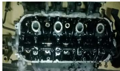
Fig. 7 Contaminates and sludge accumulated around the cylinder and engine chamber and inner oil guide
