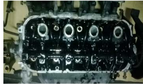
Fig. 7 Contaminates and sludge accumulated around the cylinder and engine chamber and inner oil guide
