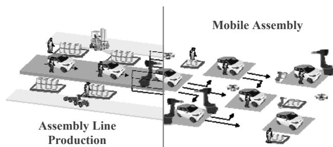
Fig. 4 Assembly line production vs. mobile assembly
