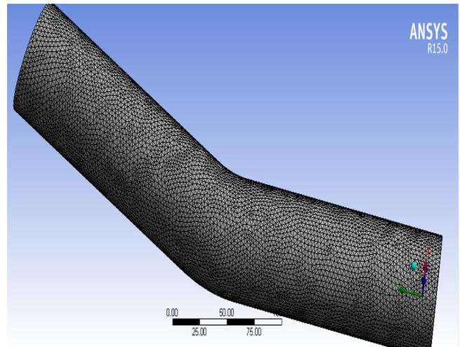
Fig. 3 Geometry and computational mesh distribution for the pipe bend model
