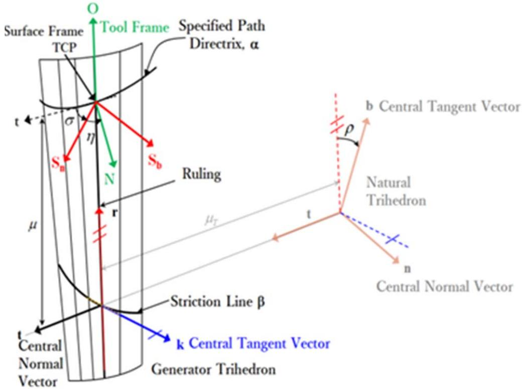
Fig. 4 Relation between surface and tool frame
