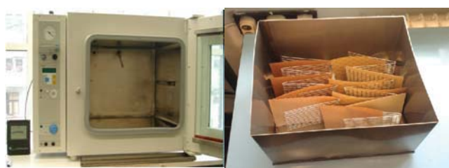
Fig. 5 The drying furnace and paper samples placed in a preformed metallic container
