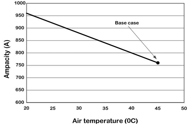
Fig. 3 Ampacity ratings versus air temperature
