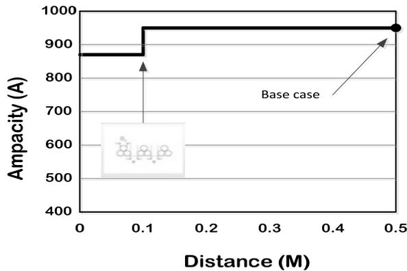
Fig. 6 Ampacity ratings versus distance between trefoils
