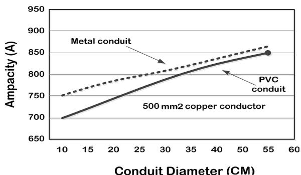
Fig. 11 Ampacity rating versus conduit diameter
