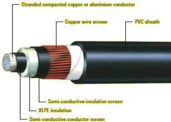
Fig. 17 Cross-sectional area for the 11KV cable
