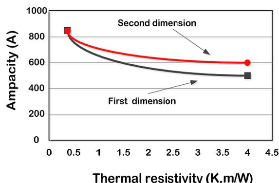
Fig. 16 Ampacity rating versus the backfill dimensions
