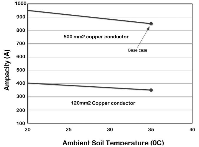
Fig. 8 Ampacity ratings versus ambient soil temperature
