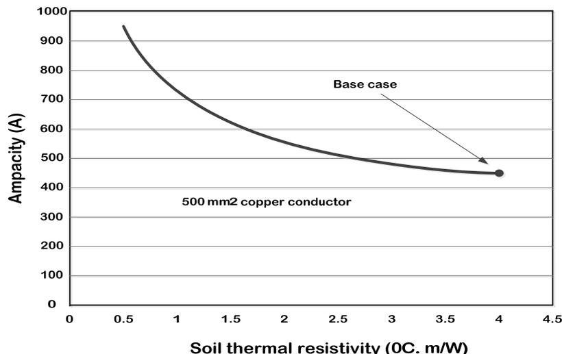
Fig. 9 Ampacity rating versus soil thermal resistivity
