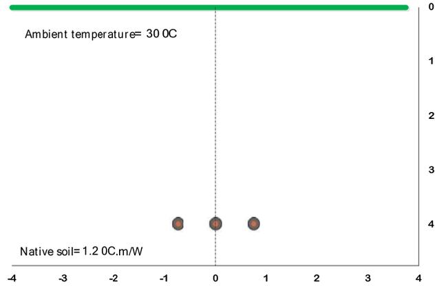
Fig. 18 Flat formation installation
