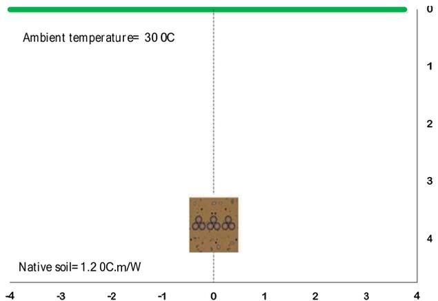
Fig. 20 Three trefoils directly buried in the soil
