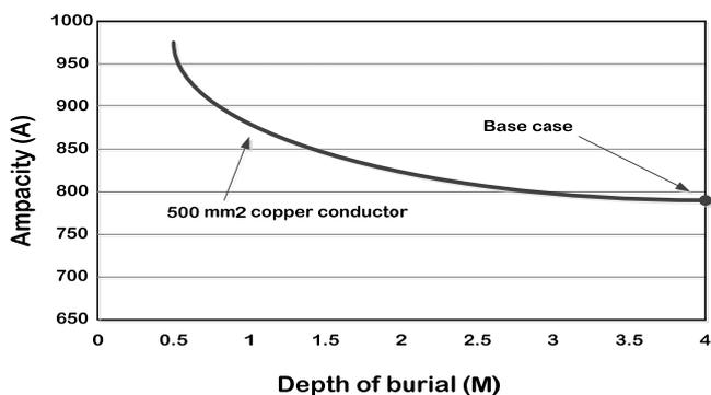
Fig. 10 Ampacity rating versus depth of burial
