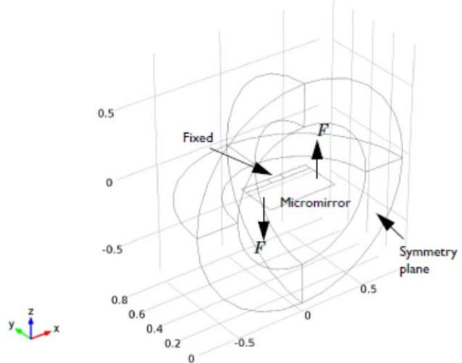
Fig. 2 Geometry of the modeled vibrating micromirror
