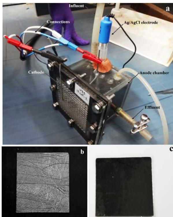
Fig. 1 Schematic design of the MFC (a) complete assembly; (b) details of anode; and (c) air-breathing cathode attached to the membrane
