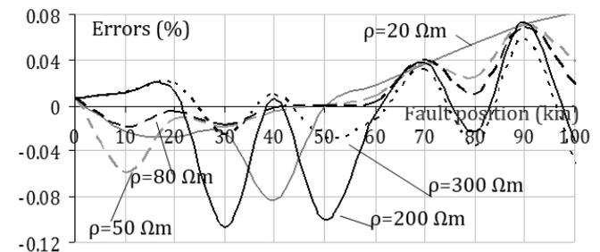
Fig. 8 Errors introduced by the two-end data algorithm
