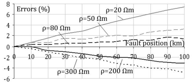
Fig. 7 Errors introduced by the one-end data algorithm
