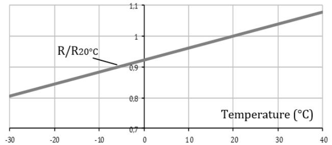
Fig. 2 Dependence of the resistance with temperature
