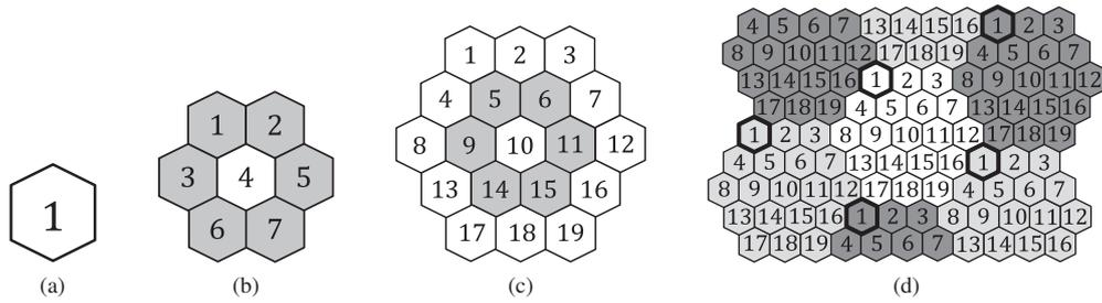
Fig. 3 Coloring by [20]: (a) 1-coloring, (b) 7-coloring, (c) 19-coloring, (d) Tessellation with 19-coloring
