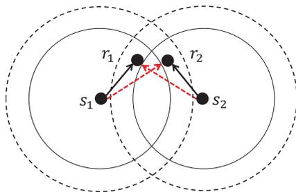
Fig. 2 Collision-Interference-Free Graph Model. Solid circles are broadcasting areas, and dotted circles are interference areas of the senders  $s_1$  and  $s_2$ . For any  $\rho > 1$ , even there is no collision occurring at any receivers  $r_1$  and  $r_2$ ,  $s_1$  and  $s_2$  cannot send data simultaneously because  $r_1$  and  $r_2$  are interfered by  $s_2$  and  $s_1$ , respectively
