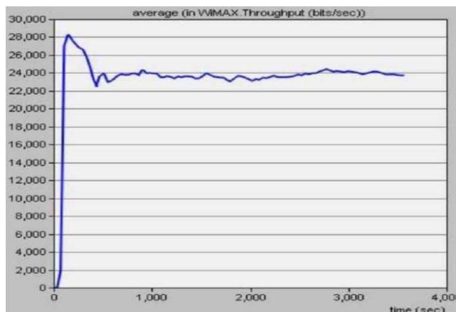
Fig. 6 Average WiMAX Throughput of Single Smart Meter
