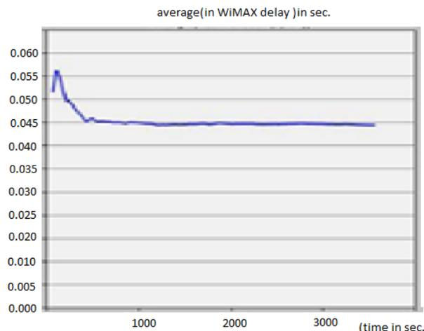
Fig. 7 Average WiMAX delay of Single smart meter
