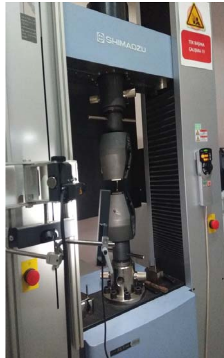
Fig. 3 Tensile testing machine (Shimadzu AG-X Plus 250 kN)
