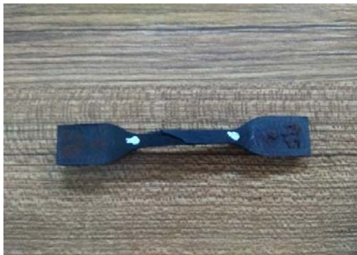
Fig. 2 Specimen is tested at 0.5 mm/s
