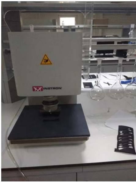
Fig. 1 Specimen preparation machine (Instron 6054.000)
