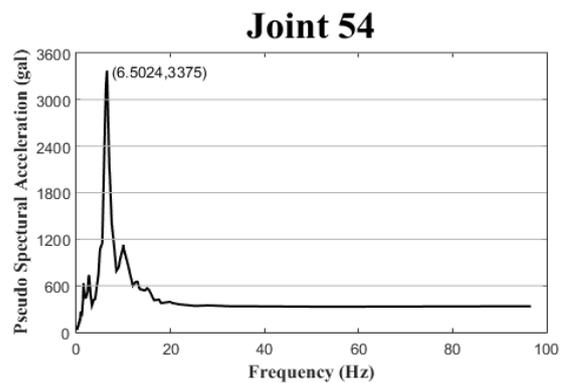
Fig. 5 The response spectrum of joint 54
