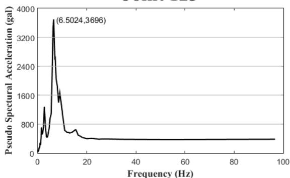
Fig. 6 The response spectrum of joint 123
