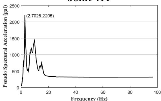
Fig. 11 The response spectrum of joint 411
