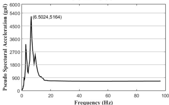
Fig. 9 The response spectrum of joint 359
