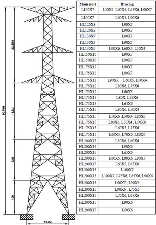
Fig. 3 The structure of the A4 EHV transmission tower
