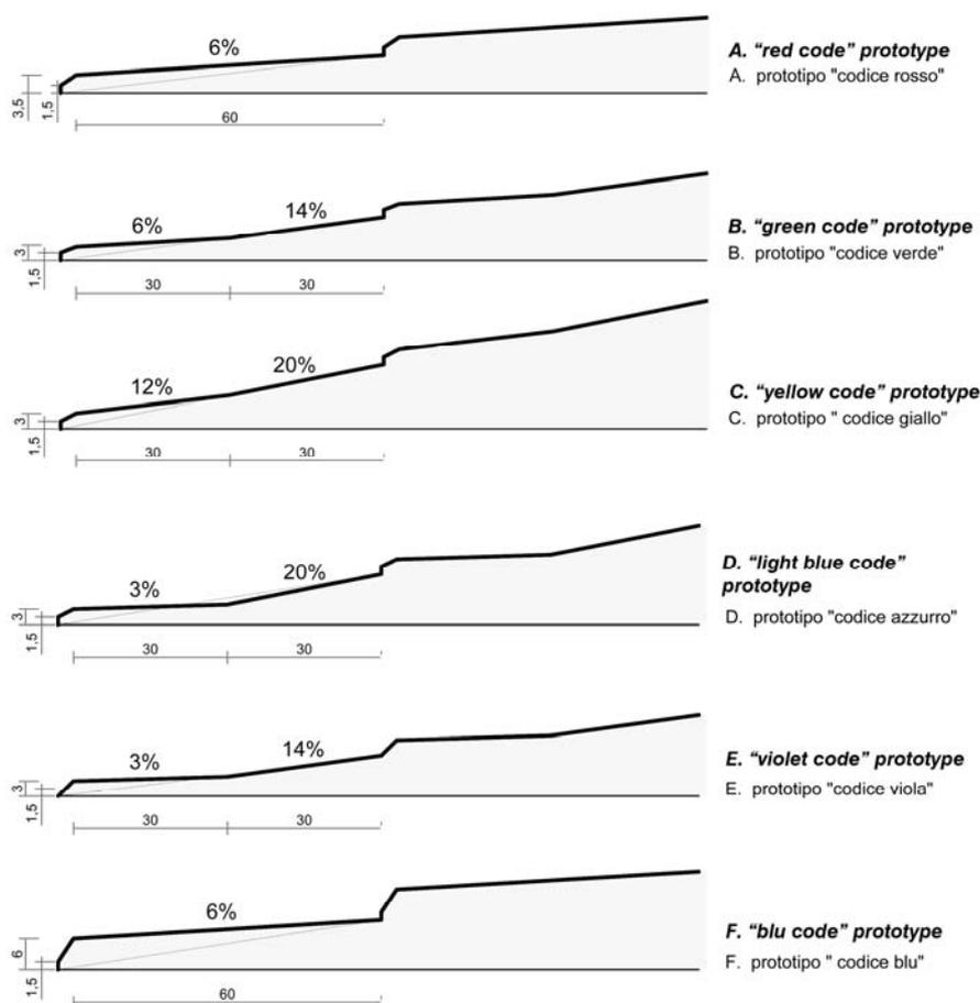
Fig. 6 Prototypes of “stepped ramp”, elaboration from the Venice Municipality study [6]
