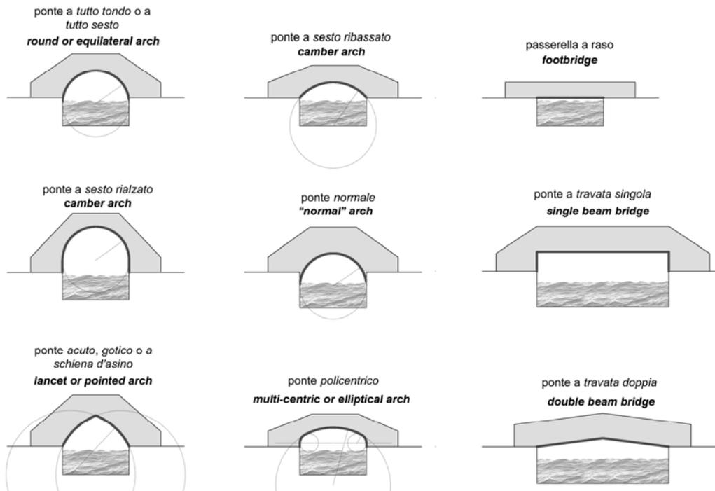
Fig. 1 Venetian bridges typologies: different geometries and structures determine the importance of considering each bridge as peculiar
