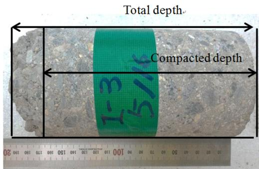
Fig. 3 Measurement of compacted depth
