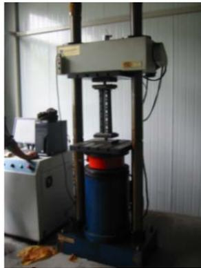
Fig. 2 The testing set-up and supporting system of EN15512 [10]
