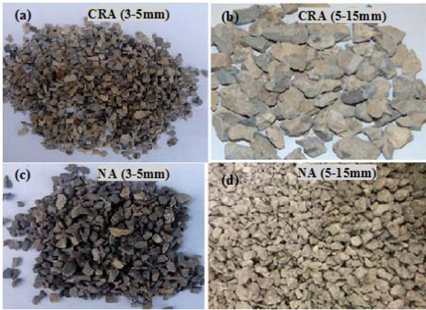
Fig. 3 (a), (b): CRA and (c), (d): Coarse natural aggregates
