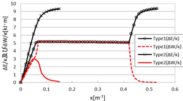
Fig. 19 Different energy characteristics in type 1 and 2
