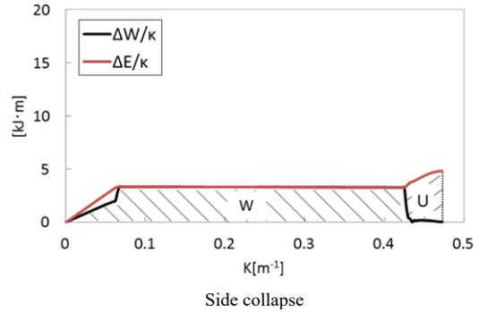
Fig. 16 Absorption energy at side collapse mode
