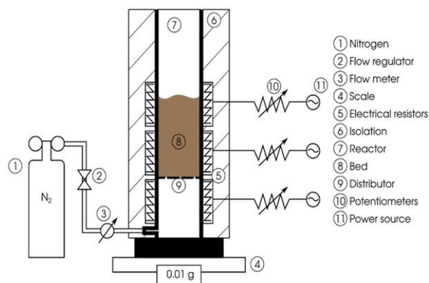
Fig. 1 Schematic illustration of the experimental facility
