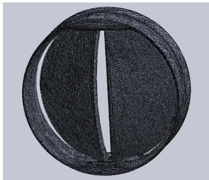
Fig. 3 Mesh from CT scanner
