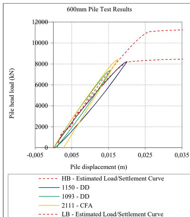
Fig. 90 600-mm estimated vs test load settlement curve
