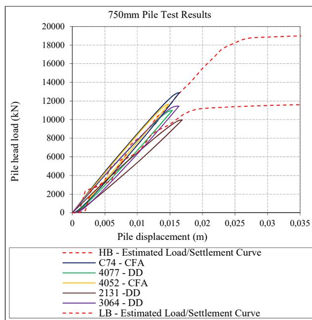
Fig. 101 750-mm estimated vs test load settlement curve
