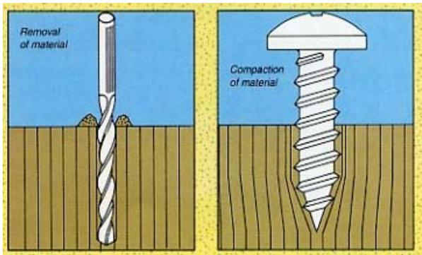
Fig. 4 Wood drill vs screw analogy as in [8], [9]
