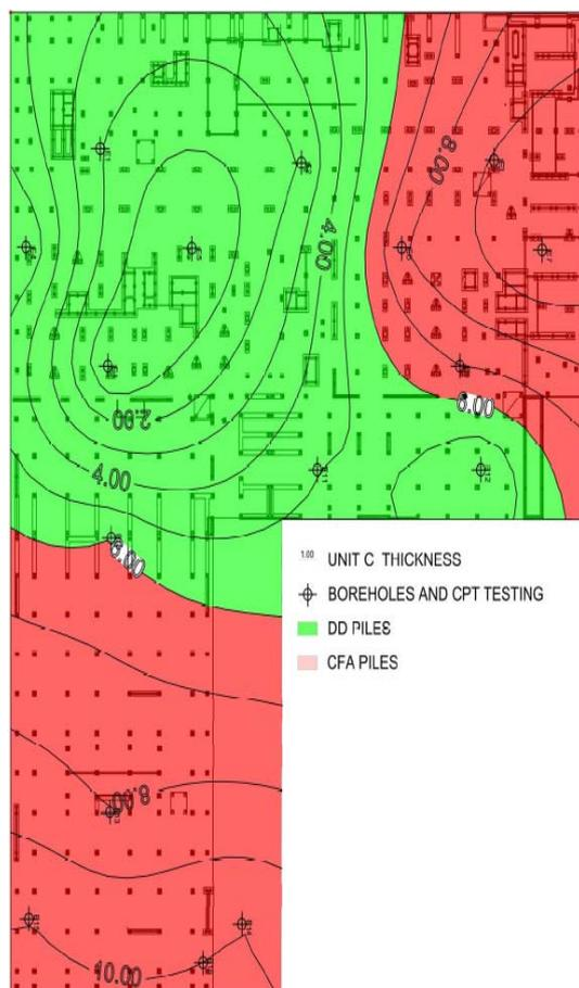
Fig. 6 Unit C thickness contours map
