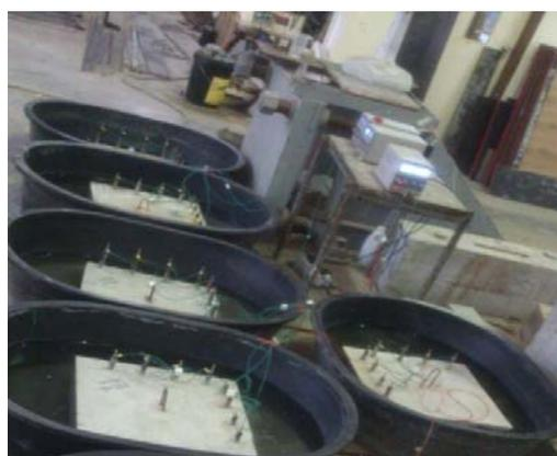
Fig. 1 Accelerated corrosion apparatus for slab elements
