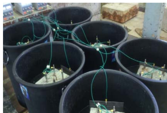
Fig. 2 Accelerated corrosion apparatus for column elements
