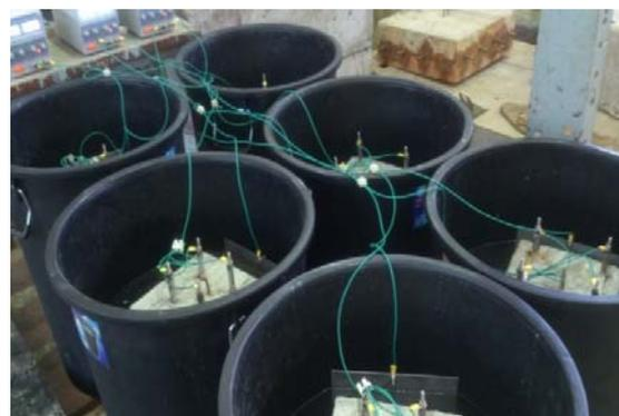
Fig. 2 Accelerated corrosion apparatus for column elements
