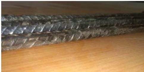
Fig. 4 Cleaned rebars after corrosion
