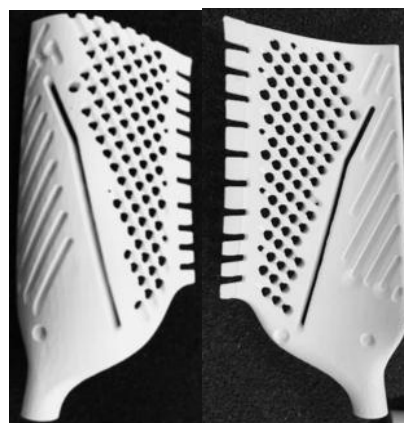
Fig. 7 Ceramic core for the blade
