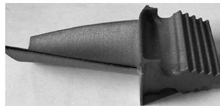
Fig. 8 The blade manufactured by DMLS technology
