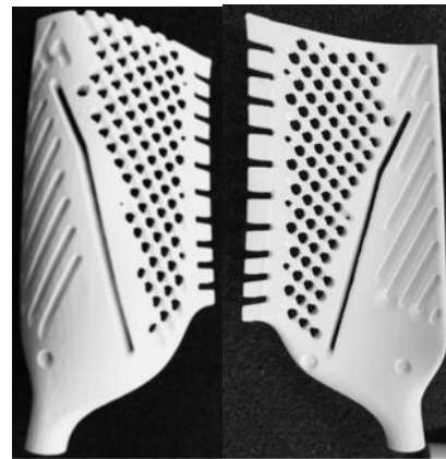
Fig. 7 Ceramic core for the blade
