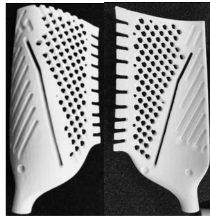
Fig. 7 Ceramic core for the blade
