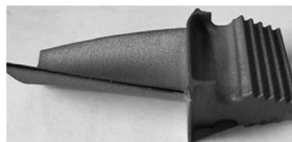
Fig. 8 The blade manufactured by DMLS technology
