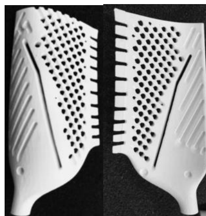
Fig. 7 Ceramic core for the blade
