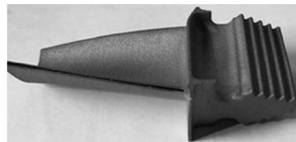
Fig. 8 The blade manufactured by DMLS technology
