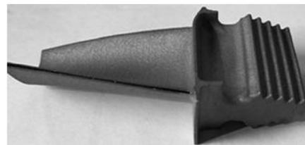
Fig. 8 The blade manufactured by DMLS technology
