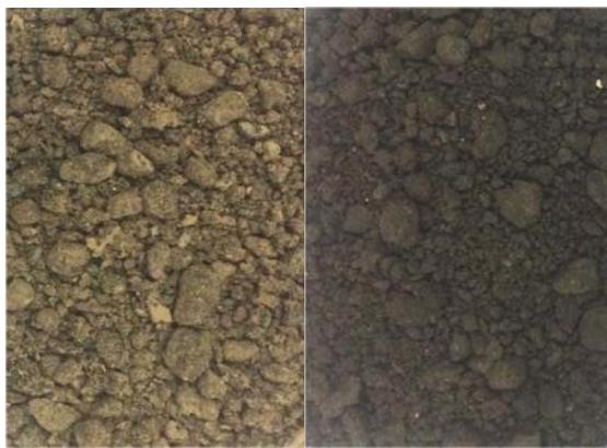
(a) Sand asphalt (b) CR-sand asphalt
