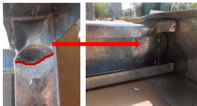
(a) Distortional bucking of W-1 CFS
