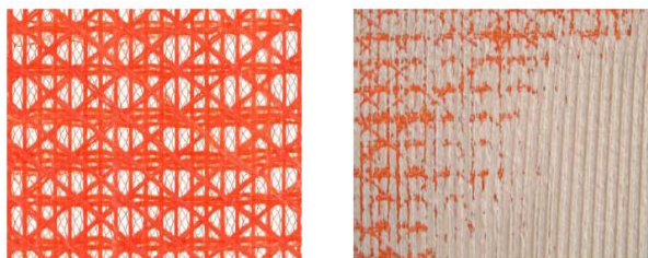
Fig. 2 The hybrid multiaxial seismic textile
