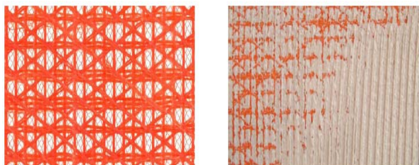
Fig. 2 The hybrid multi-axial seismic textile
