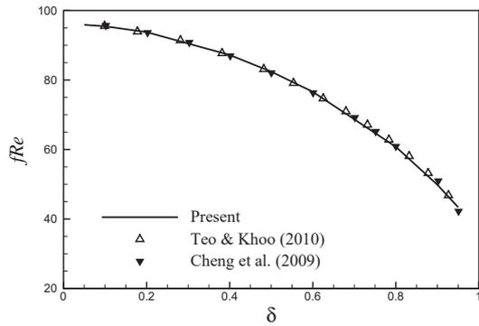
Fig. 2 Validation of numerical results in terms of friction coefficient  $fRe$  with different shear free fraction at  $L = 1$  and  $Re = 1$
