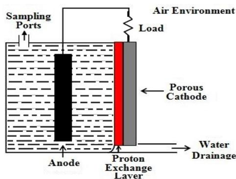
Fig. 2 Schematic diagram of the single-chamber MFC structure [10], [17], [18]
