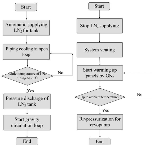
Fig. 4 Control flowchart of LN<sub>2</sub> supplying system for cryopumps
