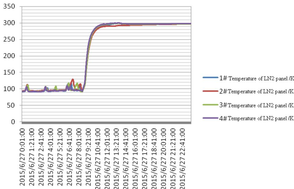
Fig. 7 Warming up curves of LN<sub>2</sub> panels in cryopumps
