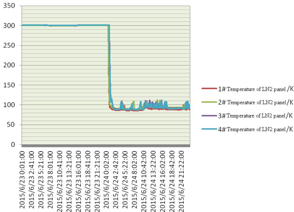
Fig. 6 Cooling down curves of LN<sub>2</sub> panels in cryopumps
