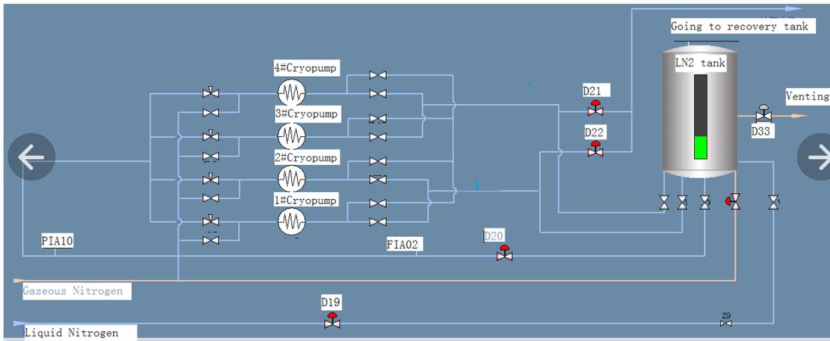
Fig. 5 Control software interface of LN<sub>2</sub> supplying system for cryopumps
