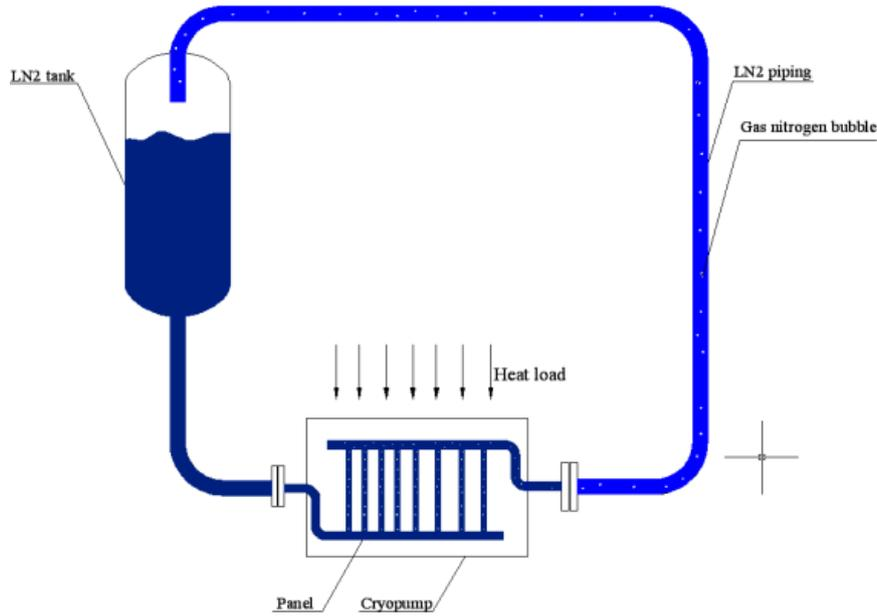
Fig. 1 Schematic drawing of gravity circulation loop system
