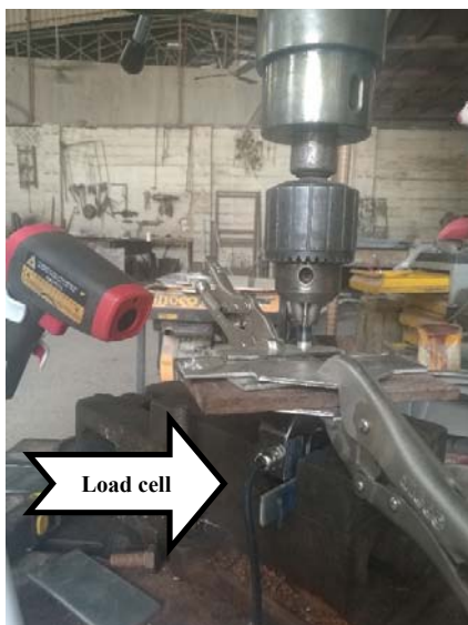
Fig. 6 Load cell and infrared temperature device arrangement
