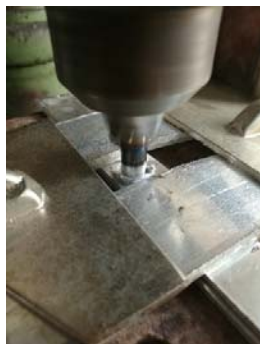
Fig. 5 Welding pin fixation in drilling holder
