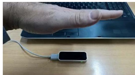
Fig. 6 Leap Motion controller use
