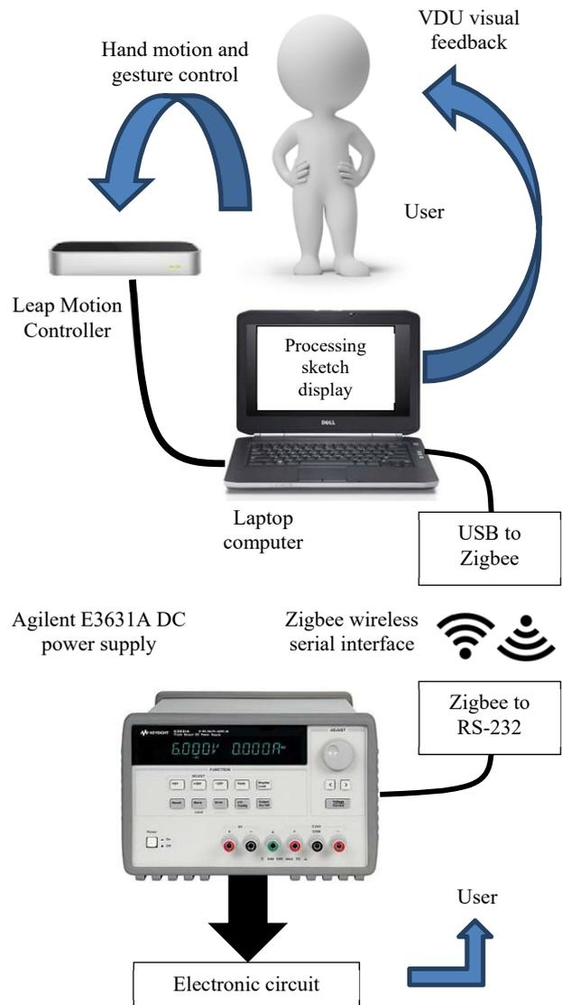
Fig. 7 Hand motion and gesture control system
