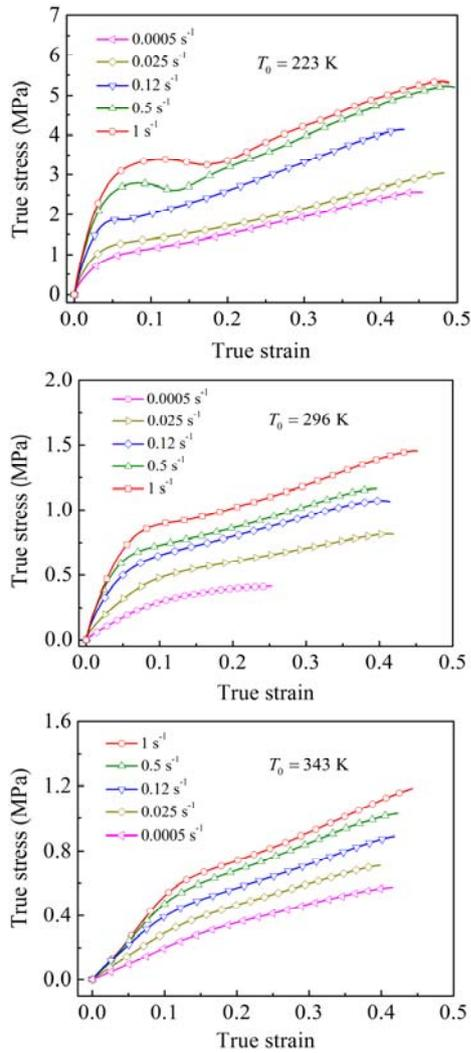
Fig. 5 Stress vs. strain curves at various temperatures
