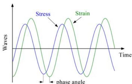
Fig. 8 The lag angle between stress and strain
