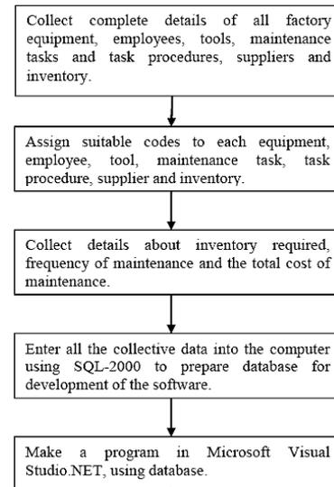
Fig. 2 Phases for developing CMMS
