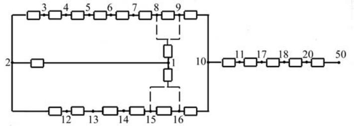
Fig. 5 The equivalent hydraulic scheme of experimental nozzle blade cooling system
