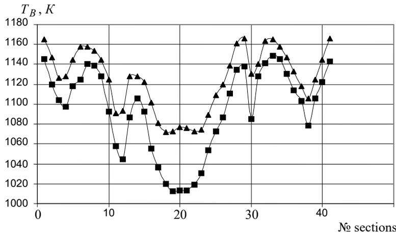
Fig. 6 Distribution of temperature along outside (▲) and internal (■) contours of the cooled nozzle blade
