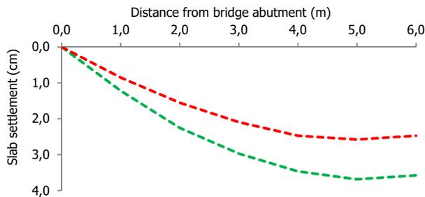
Fig. 5 Settlements calculate analytically, Green line shows the settlement when soil subgrade reaction is taken 24.000 kN/m<sup>3</sup>, Red line shows the settlement when soil subgrade reaction is taken 32.000 kN/m<sup>3</sup>
