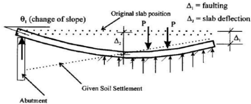
Fig. 2 The model of bridge approaching slab under given embankment settlement [8]
