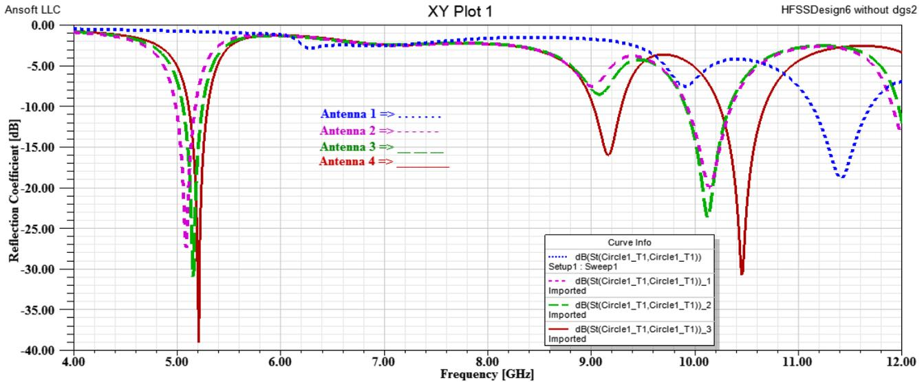
Fig. 5 Return loss comparison
