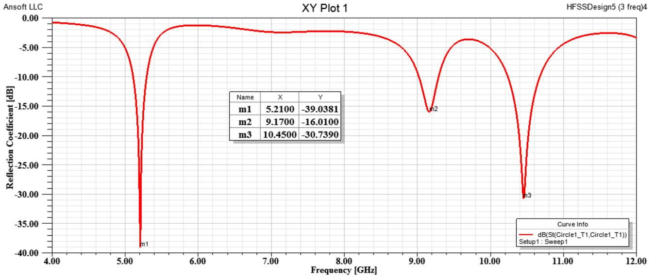
Fig. 7 S-parameter for the Proposed Model
