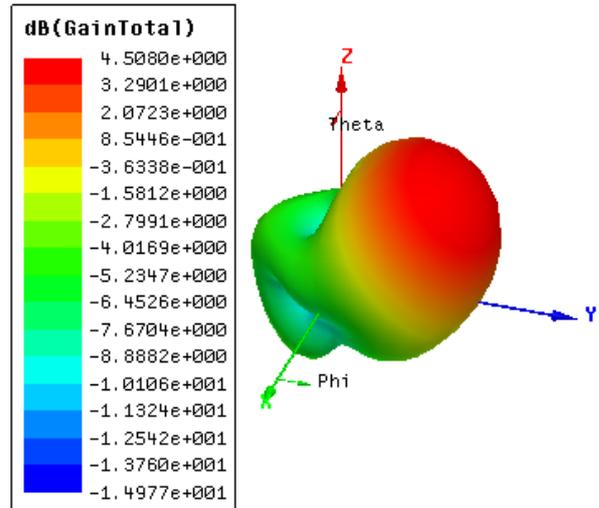
Fig. 12 Gain at 9.17 GHz
