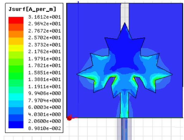
Fig. 10 Current Distribution at 10.45 GHz
