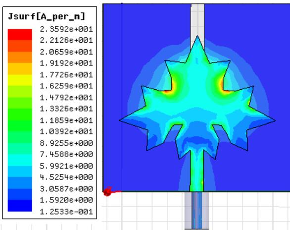
Fig. 8 Current Distribution at 5.21 GHz
