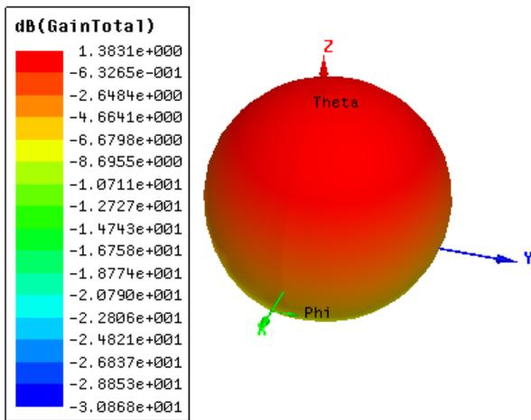
Fig. 11 Gain at 5.21 GHz
