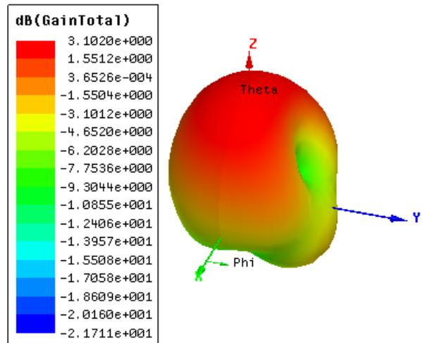
Fig. 13 Gain at 10.45 GHz
