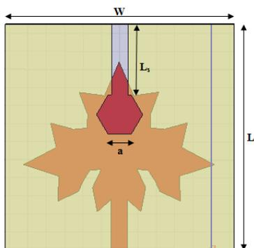
Fig. 3 Proposed Design Model – view from bottom
