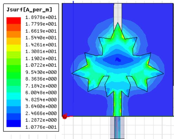
Fig. 9 Current Distribution at 9.17 GHz
