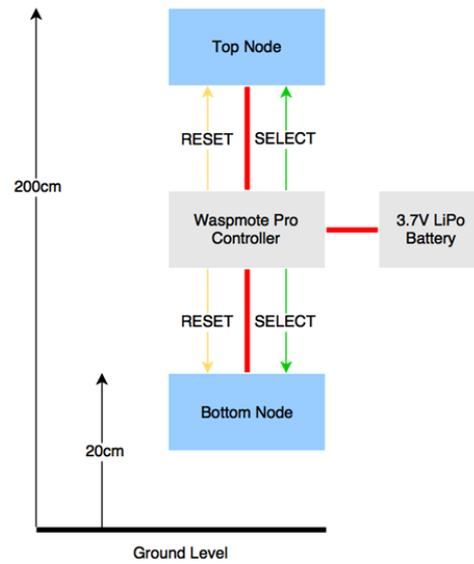
Fig. 4 Block diagram of range test apparatus
