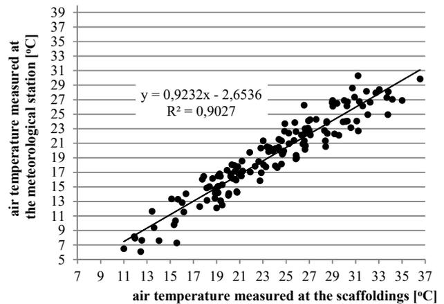
Fig. 5 The dependence of the values of the air temperature measured at the meteorological station and at scaffoldings
