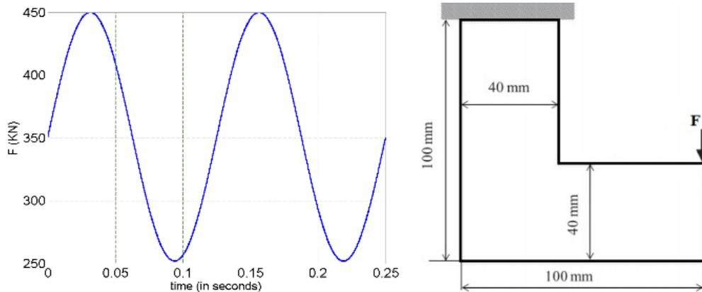
Fig. 2 Design domain, loading and boundary conditions of the L-beam
