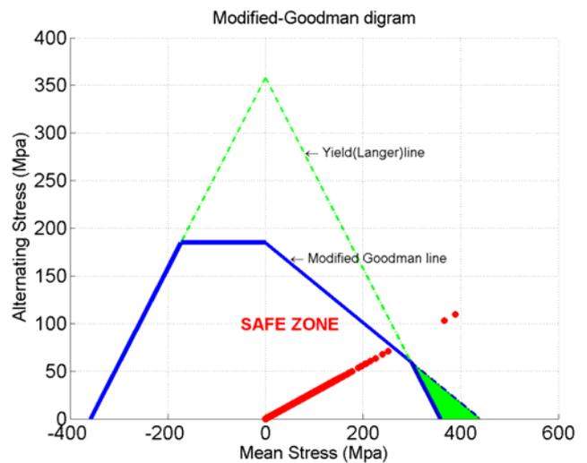
Fig. 5 Goodman fatigue diagram for compliance case
