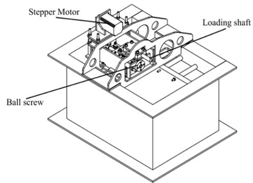
Fig. 1 Sketch of lateral loading setup
