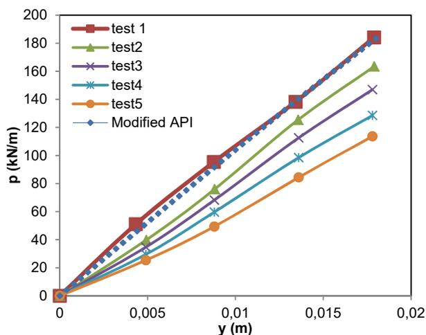
Fig. 10 Experimental and API p-y curve at  $z=3D$
