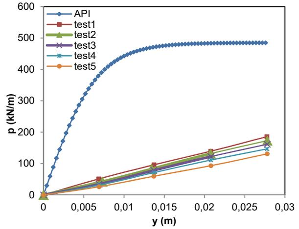
Fig. 7 Experimental and API p-y curves at z=2D
