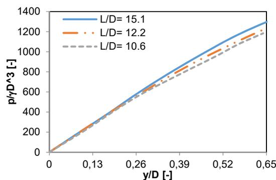
Fig. 3 Effect of embedded depth on soil (non-dimensional)
