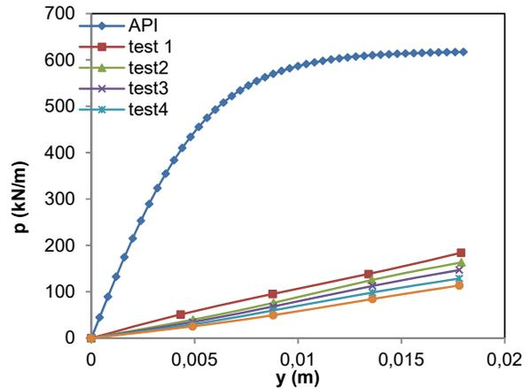
Fig. 8 Experimental and API p-y curves at z=3D
