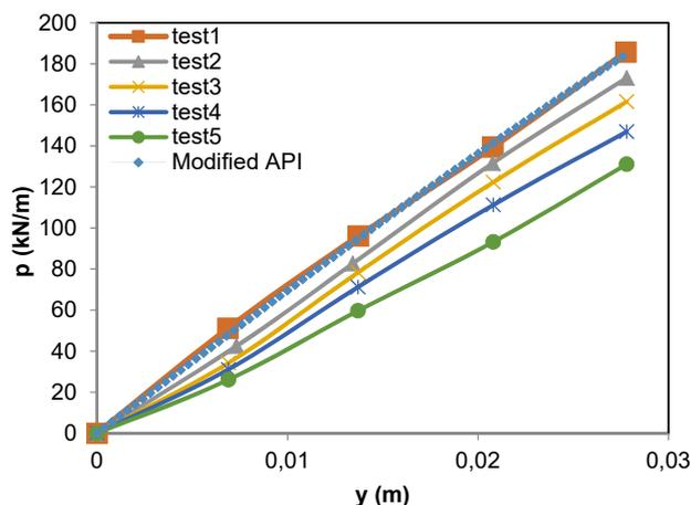
Fig. 9 Experimental and API p-y curve at  $z=2D$
