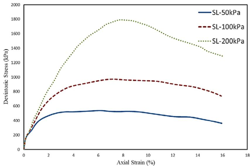
Fig. 9 Deviatoric stress versus axial strain for SL
