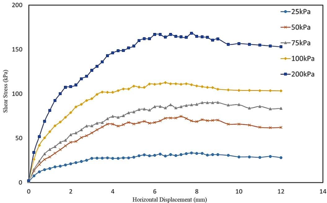
Fig. 2 Variation of shear stress with horizontal displacement for OL in loose condition
