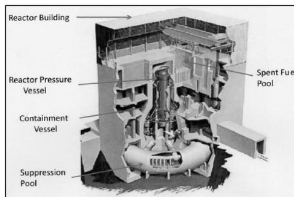
Fig. 1 Schematic Diagram of BWR in Fukushima-1 NPP [2]
