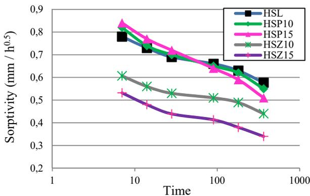
Fig. 15 Sorptivity coefficients of the studied HSSCCs at different curing ages (mm/h<sup>0.5</sup>)
