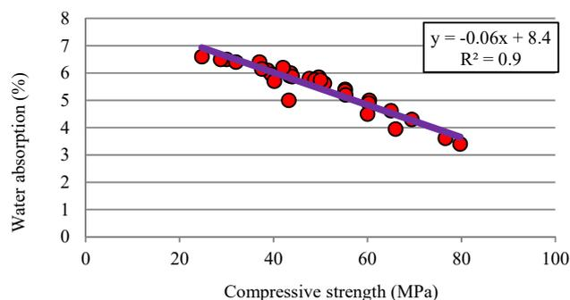
Fig. 12 Relationship between water absorption and compressive strength
