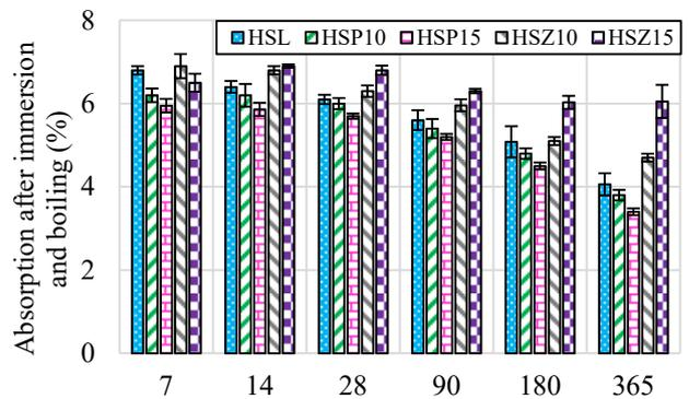
Fig. 10 Absorption after immersion and boiling (%) of studied HSSCCs
